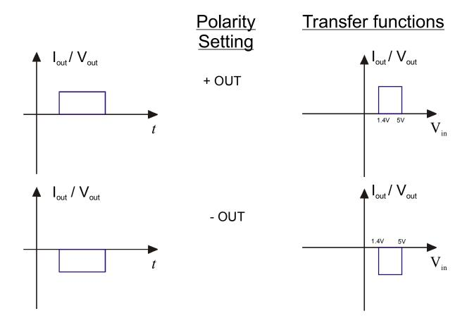
Input is Logic high (5V) or low (0V) and is TTL or CMOS compatible.
